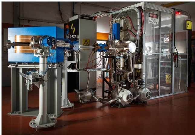
Turnkey Filament-Powered Ion Source Including Optional Beamline and Mass Spectrometer
